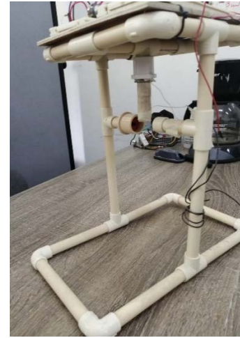
Fig. 5. PVC structure of the levitation system.
